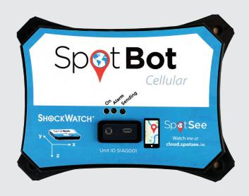
SpotBot is a standalone device that delivers tri-axial impact monitoring and tracking through cellular connectivity. It features real-time visualization through the SpotSee web based platform. You can access your data in the cloud from any web-based device. The SpotBot transmits information using cellular technology, so the unit does not require line of sight to a satellite for position or communication.
