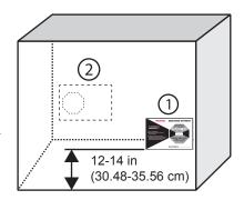
B. If the package is twice as long as it is wide, or palletized shipments use two ShockWatch labels.
